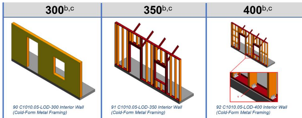
Figure 3: Sample images of Cold Formed Metal Framing (CFMF) from BIMForum Global specification. Note that at LOD 350 only studs are modeled, whereas connection fasteners are included at LOD 400.
