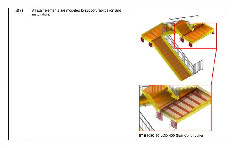
B1080.20 21-02 10 80 10 Precast Structural Stairs (Concrete)
