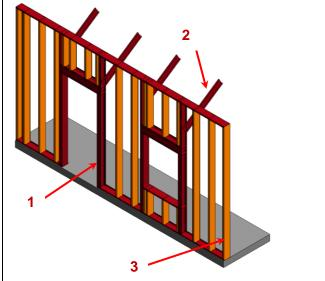
97 C1010.05-LOD-350 Interior Wall (Cold-Form Metal Framing)
