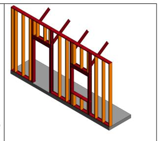
79 B2010.05-LOD-350 Exterior Wall (Cold-Form Metal Framing)
