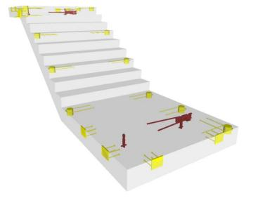
55 B1080.10-LOD 350 Precast Structural Stairs (Concrete)
