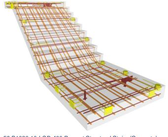
56 B1080.10-LOD 400 Precast Structural Stairs (Concrete)
