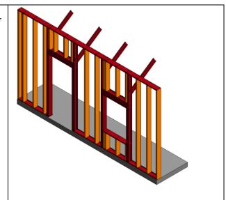
73 B2010.05-LOD-350 Exterior Wall (Cold-Form Metal Framing)
