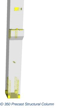
20 B1010.10 - LOD 350 Precast Structural Column (Concrete)
