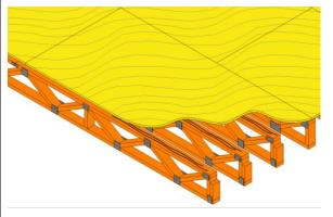
43 B1010.10-LOD-350 Floor Structural Frame (Wood Floor Trusses)
