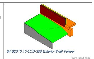
350 Exterior wall veneer modeled as a separate element.
